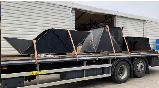
Chute sections to make up a full arrangement ready for site service installation.
