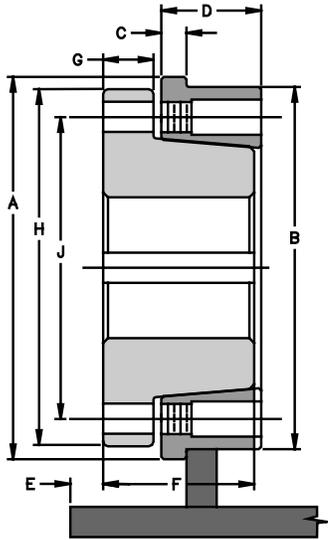
QD® has a primary benefit of bushing interchangeability with other shaft mounted components. Its shallow taper provides a high mechanical advantage to assure dependable clamping to the shaft.
